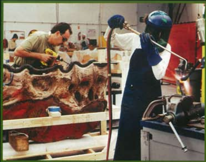
Figure 4. Lead fabricator Paul Zawisha attaches a cast of the upper pelvis of a T. rex to a metal armature while fabricator Donna Lopp bends a piece of metal tubing that will become the armature for a section of the spine. Photo courtesy of Phil Fraley Productions.
